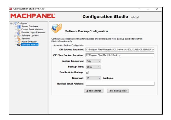
You can take backup of Control Panel and SQL database at specified locations and interval (Frequency & Time). Apply required setting and click on "Update Settings". You can enable Auto-Backup option and change Backup frequency and the backup location as well. Also, you can auto-purge backups by selecting Keep Last (Select numbers) and also you can provide Backup Email Address.
